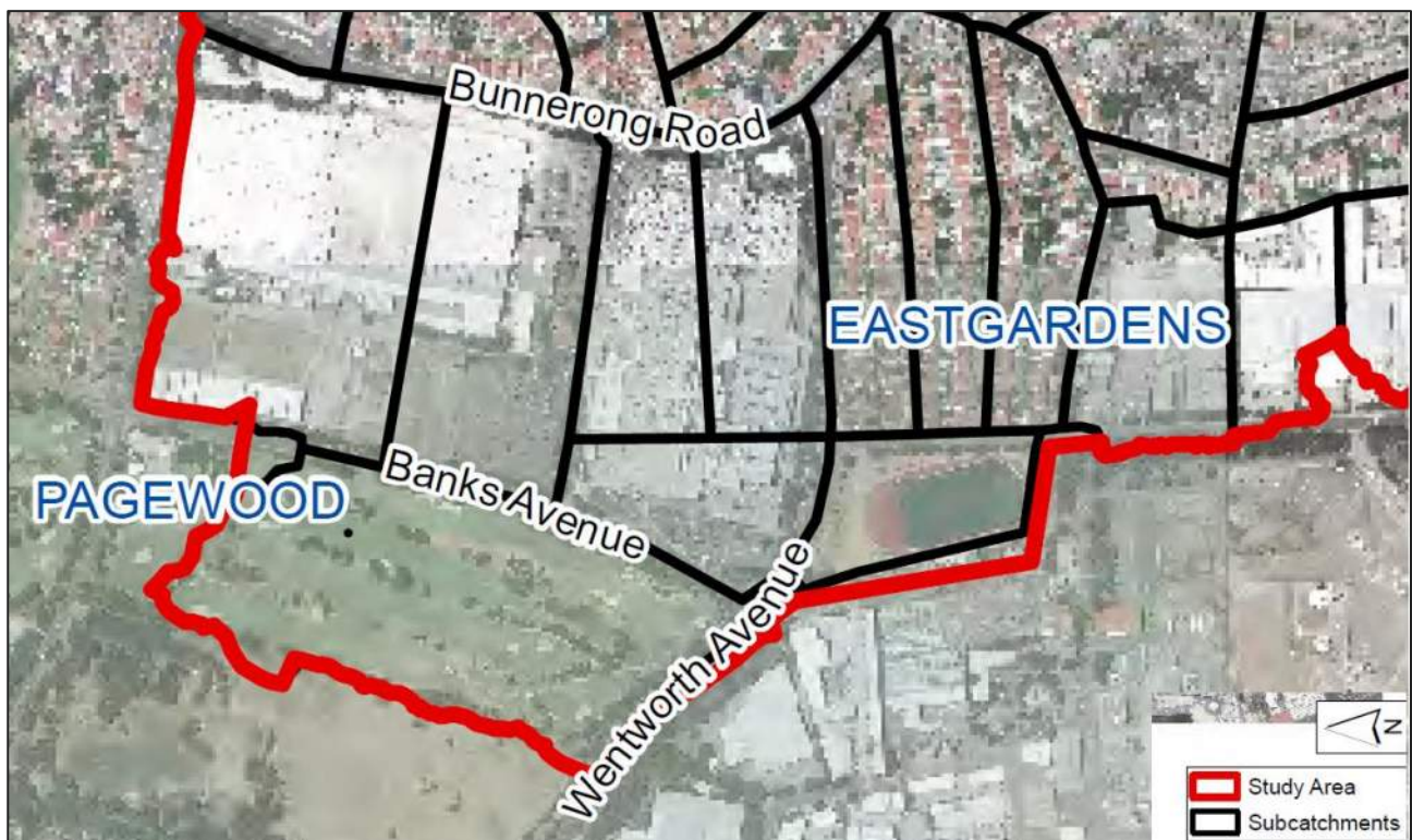
Figure 4-1 Hydrology Sub-Catchments from Flood Study (Source: WMA flood study report 2018)
